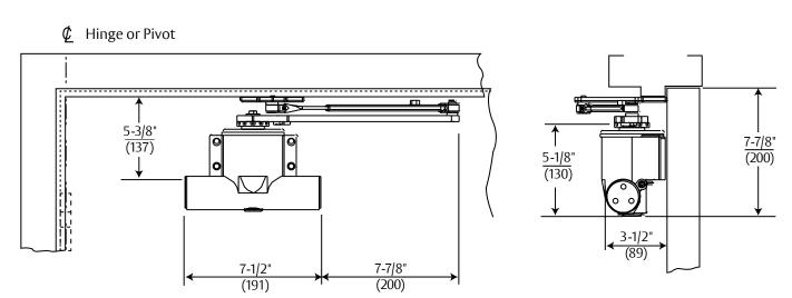
Body mounting holes are spaced 4-1/8" (105mm) horizontally and 1-3/8" (76mm) vertically.
